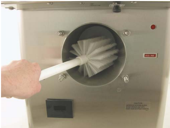
Figure 3-5 Cleaning Freezing Cylinder
