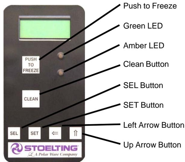
Figure 3-2 IntelliTec Control
