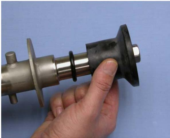
**Figure 3-5 Rear Seal Assembly**
