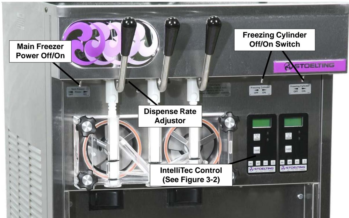
Figure 3-1 Machine Controls
