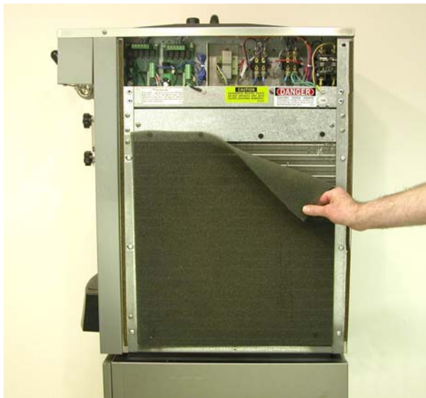
Figure 4-5 Condenser Filter Removal
