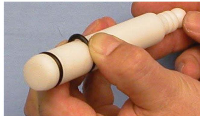
**Figure 3-4 Removing O-Ring**
