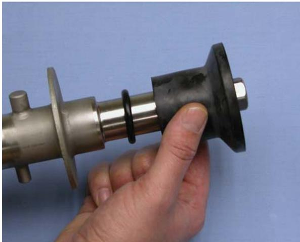
Figure 3-5 Rear Seal Assembly
