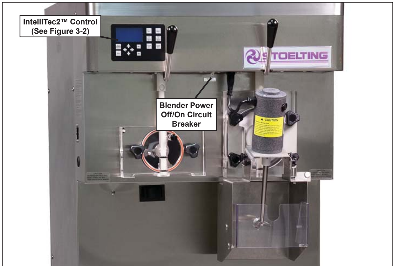
Figure 3-1 SU444 Freezer Controls
