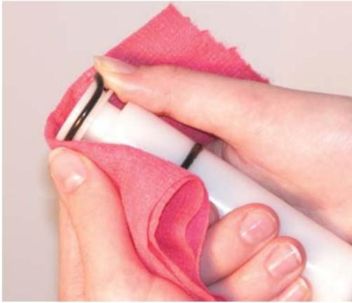
**Figure 3-4 Removing O-Ring**
