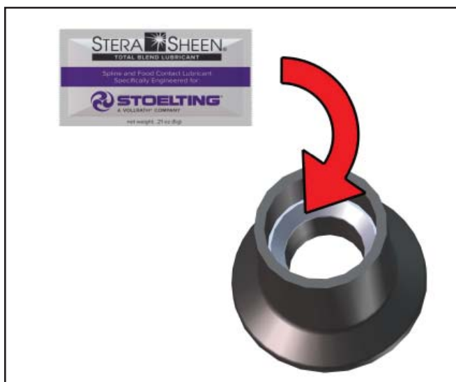
Figure 3-6 Lubricate Rear Seal
