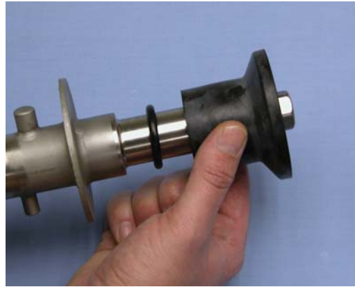
Figure 3-5 Rear Seal Assembly
