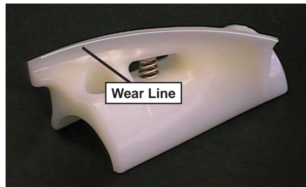
Figure 3-3 Auger Flight Wear
