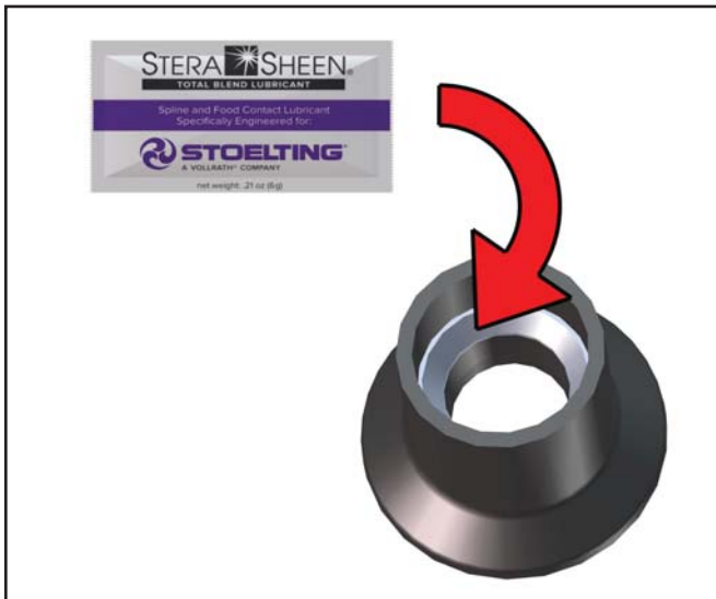
Figure 3-6 Lubricate Rear Seal
