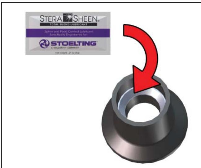
Figure 3-6 Lubricate Rear Seal
