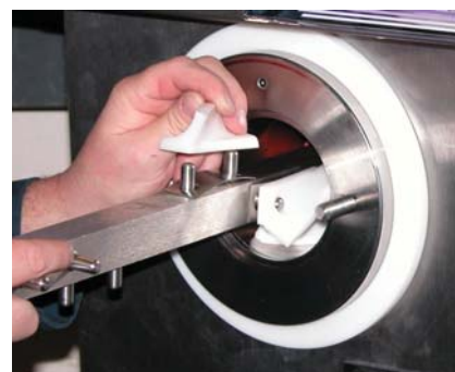
Figure 3-6 Installing Auger Blades
