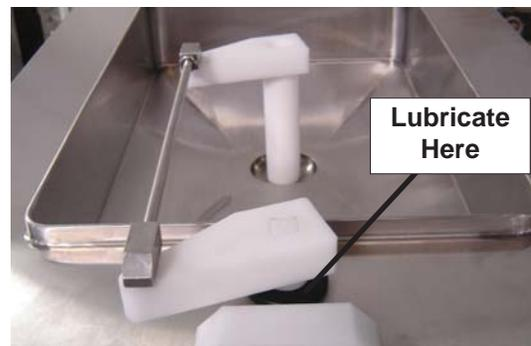
**Figure 3-6 Flow Control Arm Lubrication**
