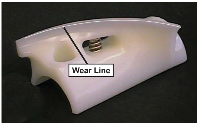
Figure 3-3 Auger Flight Wear
