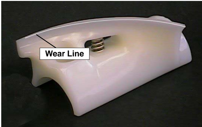
Figure 3-6 Auger Flight Wear
