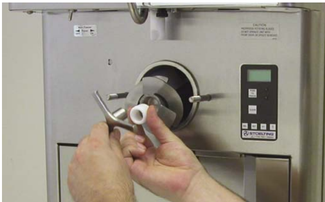
Figure 3-7 Removing Auger Support
