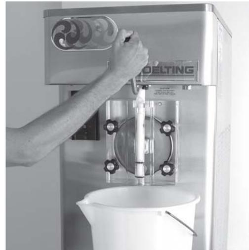
**Figure 10. Draining Solution**
