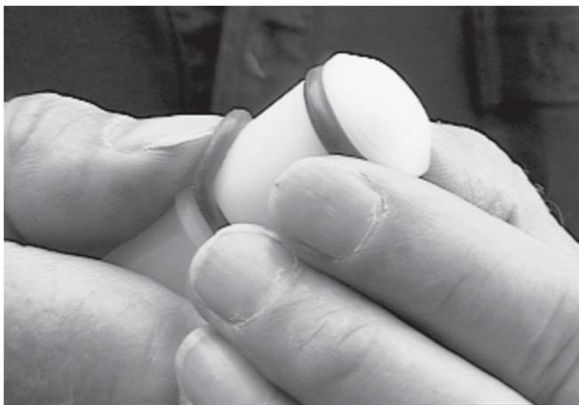
**Figure 16. Removing O-ring**
