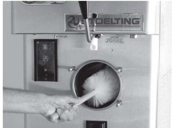
**Figure 17. Cleaning Freezer Barrel**
