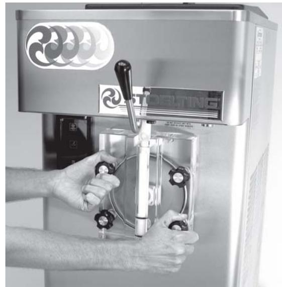
**Figure 14. Removing Front Door**
