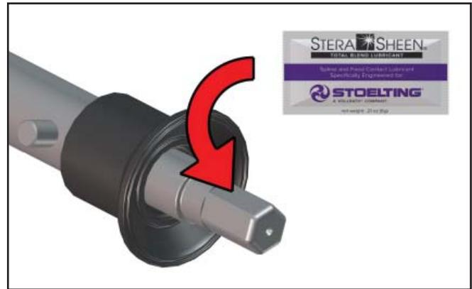
**Figure 3-6 Lubricate Hex End of Auger**
