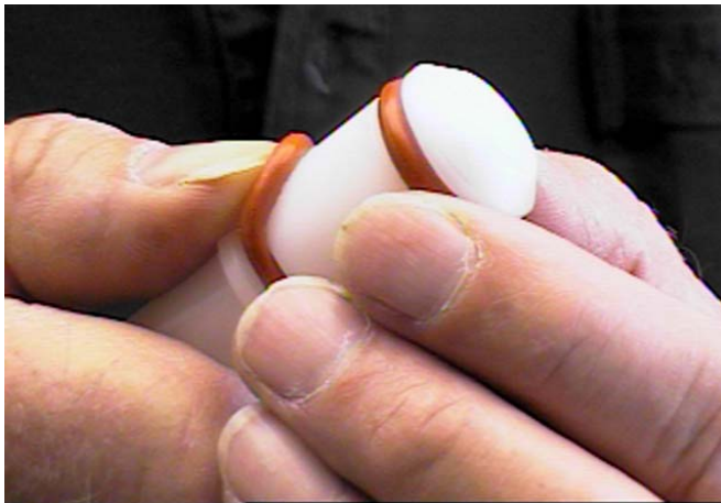
Figure 19. Removing "O" Ring
