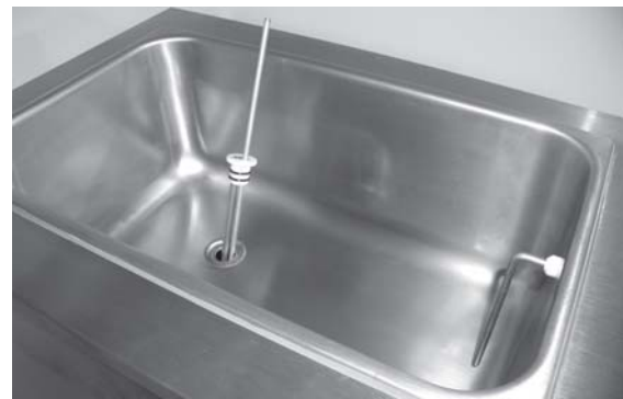
Figure 15. Removing Mix Inlet Regulator (Shown with no mix in hopper)
