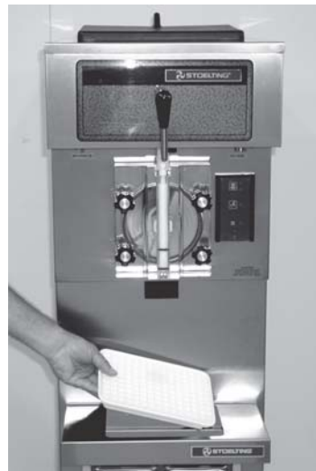
Figure 7. Installing Tray and Cover
