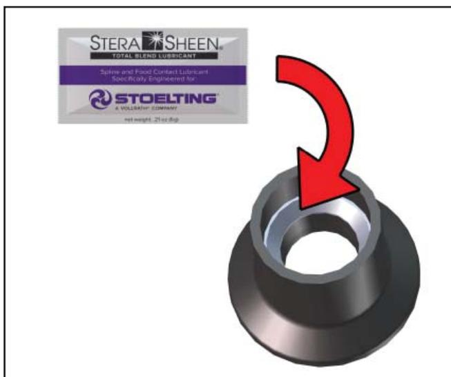
Figure 3-6 Lubricate Rear Seal
