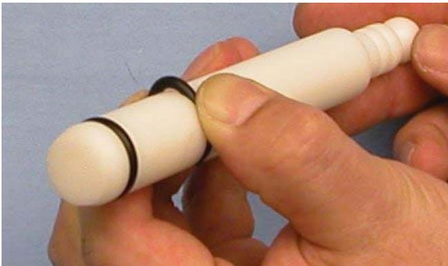
**Figure 3-4 Removing O-Ring**
