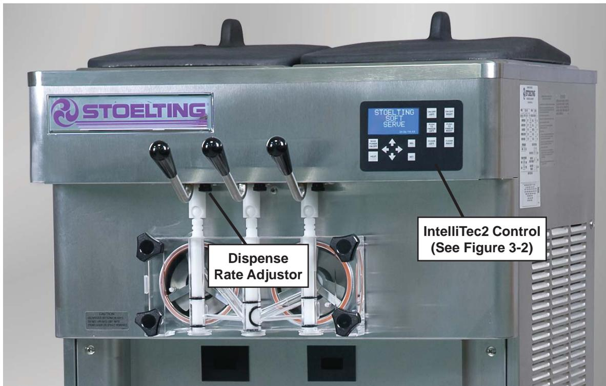
Figure 3-1 Machine Controls
