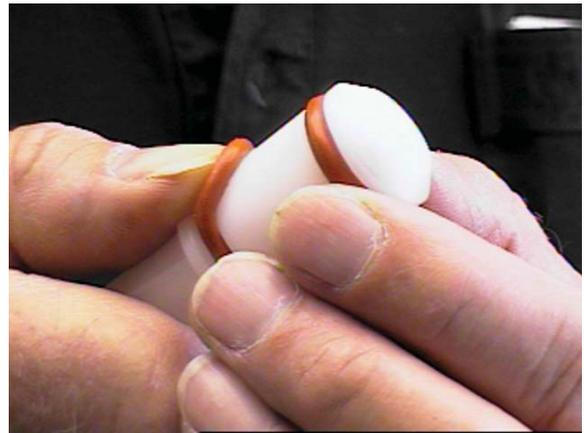
**Figure 3-4 Removing O-Ring**
