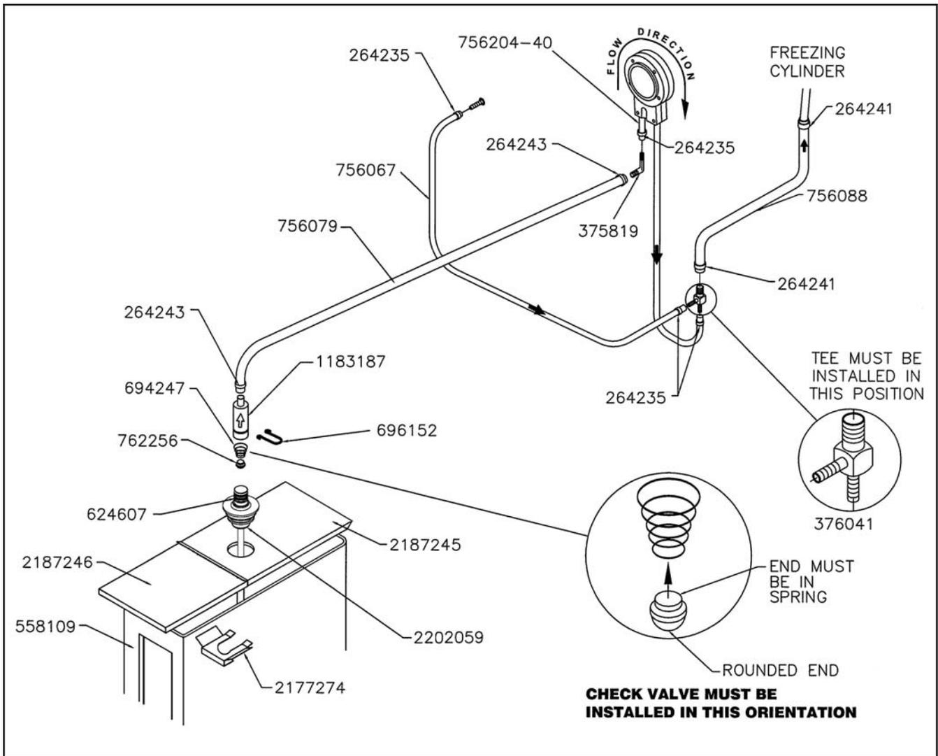
**Figure 2-3 Mix Pump Connections for Standard Mix Container**
