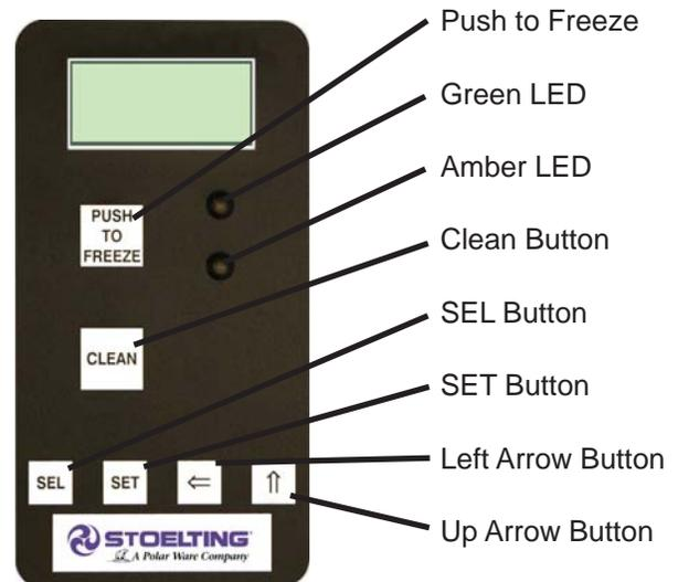
Figure 3-2 IntelliTec Control
