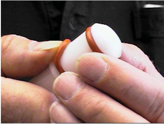
**Figure 3-4 Removing O-Ring**
