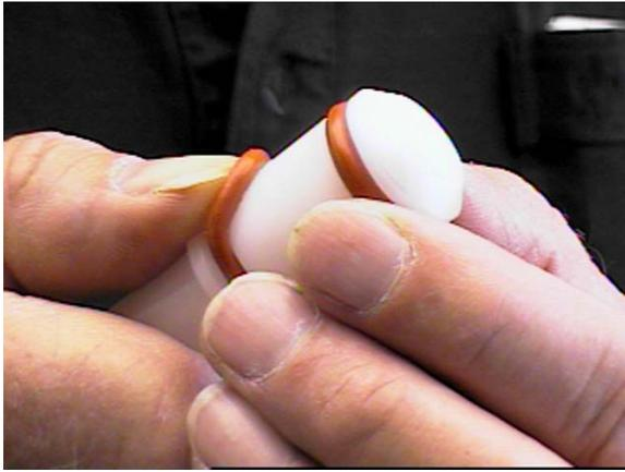
**Figure 3-4 Removing O-Ring**
