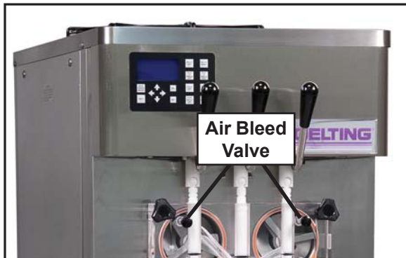
Figure 3-8 Air Bleed Valve
