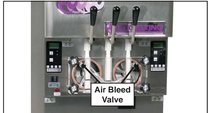
Figure 3-8 Air Bleed Valve
