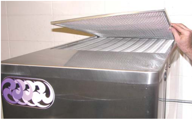
Figure 4-4 Removing Condenser Filter
