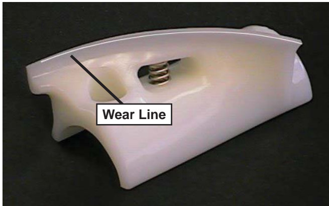
Figure 3-3 Auger Flight Wear
