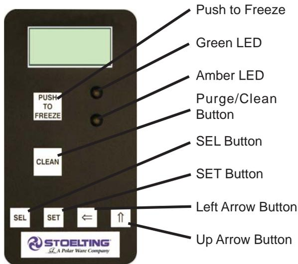
**Figure 3-2 IntelliTec Control**
