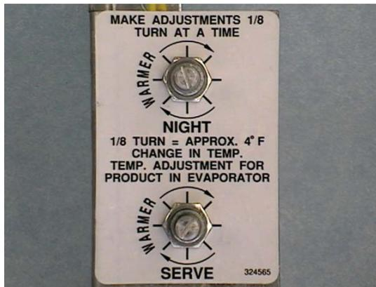
Figure 4-1 Left Side Product Temperature Control
