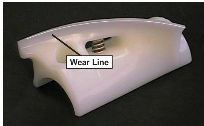
Figure 3-3 Auger Flight Wear
