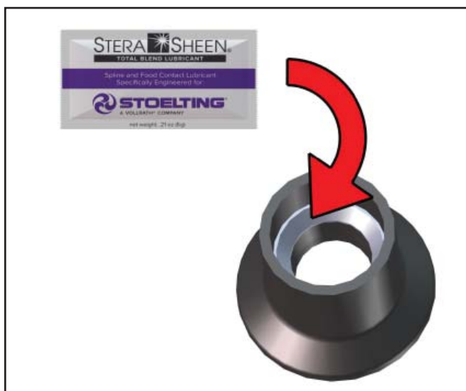
Figure 3-6 Lubricate Rear Seal
