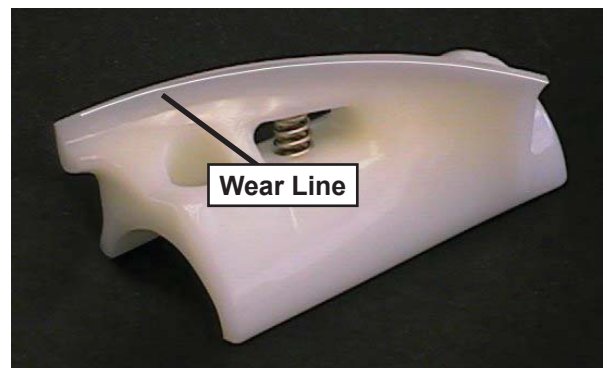
Figure 3-3 Auger Flight Wear
