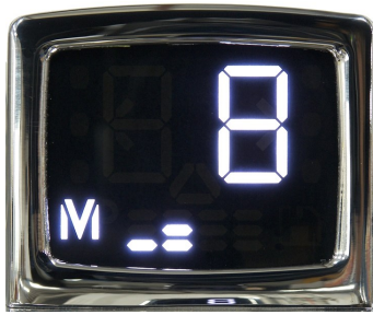
2 Bars: Bypass Pressure Ramp Up
