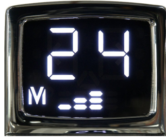
3 Bars: Pump Pressure Full Pressure Brew (9 bar)
