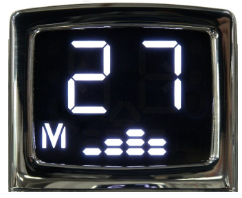
2 Bars: Bypass Pressure Ramp Down
