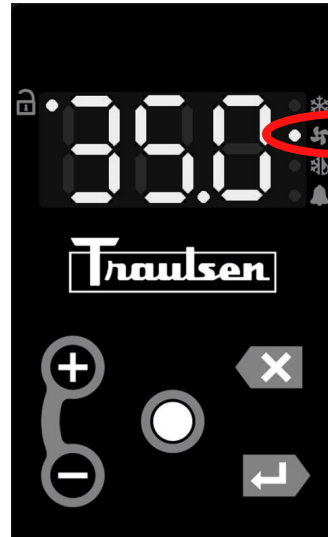
Fig. 4.4b ONLY Fan Icon Illuminates with Off-cycle Defrost
