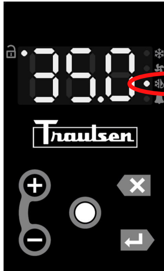
Fig. 4.4a Defrost Icon Illuminates in electric Defrost ONLY
