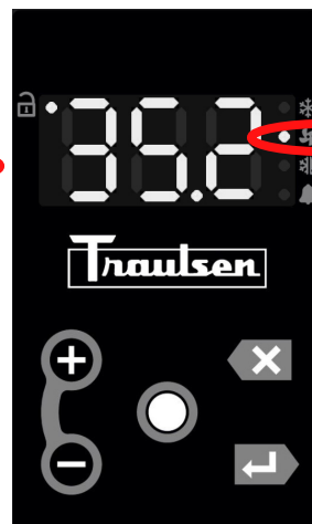
Evap Fan On
