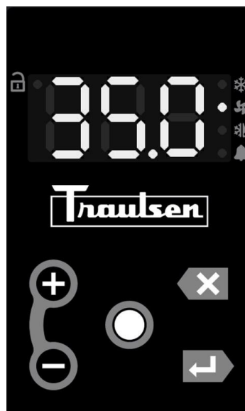
Fig. 6B.15.2a Display During Off-cycle Defrost
