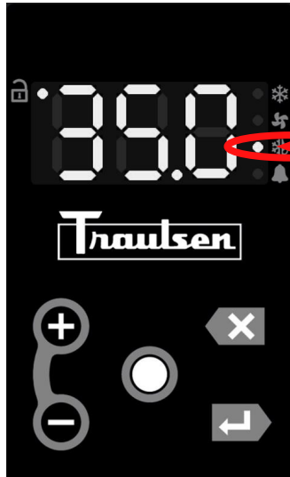
Fig. 4.4a Defrost Icon Illuminates In Electric Defrost ONLY
