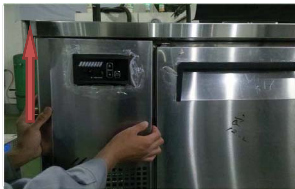
C. Remove the mech cover
