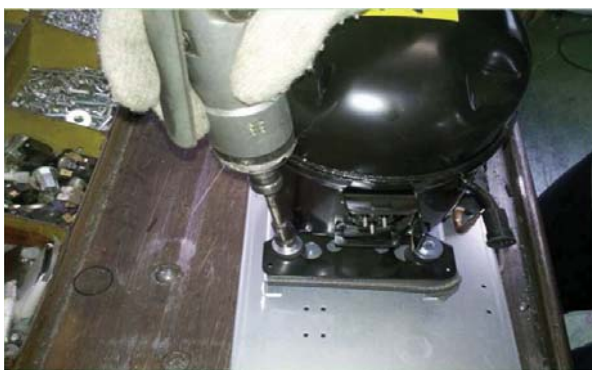
E. Unscrew the condenser.
