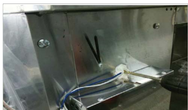
L . Disconnect the harness sensor.
