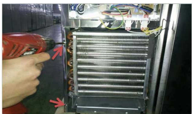
D. Remove the comp base
