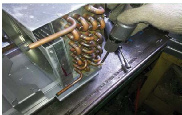
E. Unscrew the condenser.
