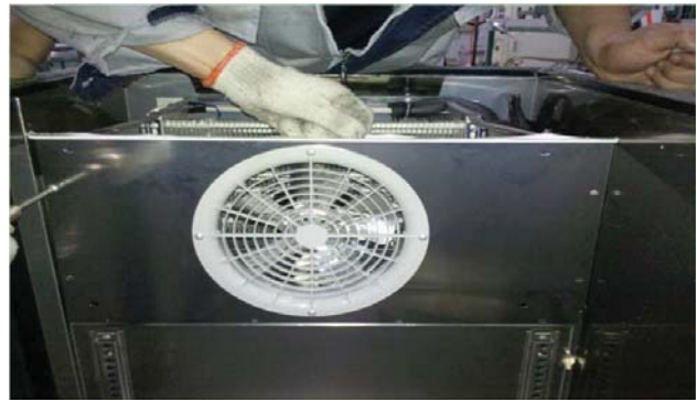
H.Disassemble evap motor.
