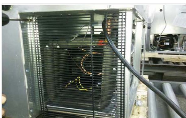
C. Remove the mech cover
