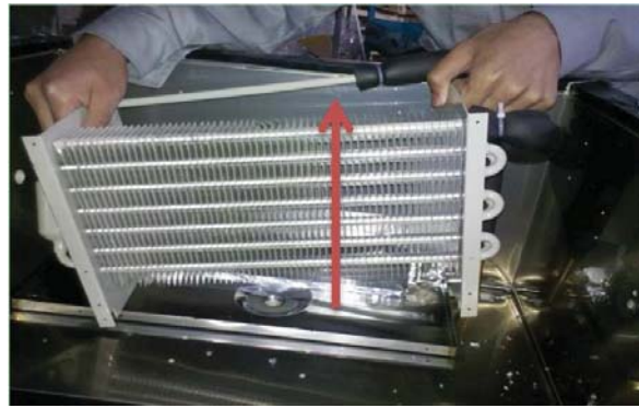
O. After unscrewing, remove evaporator.
