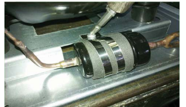
F. Disassemble filter dryer.
