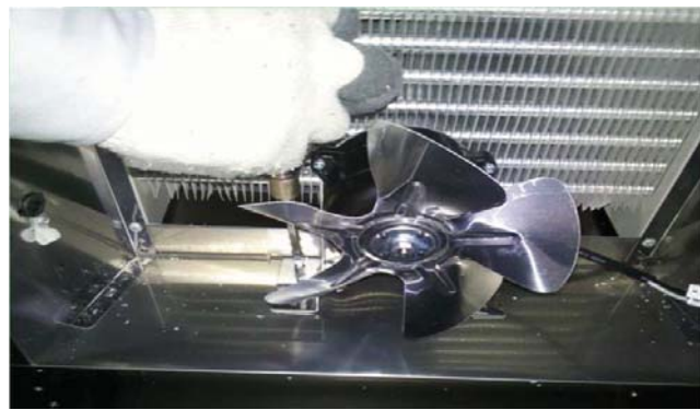
J.Disassemble air guide
