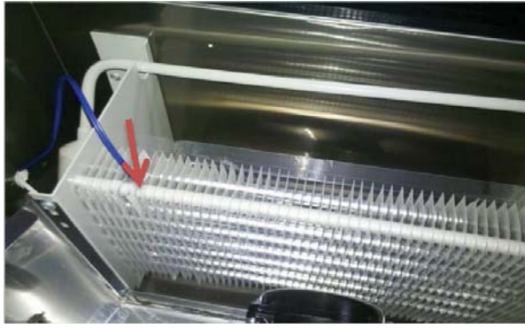
O. After unscrewing, remove evaporator.
