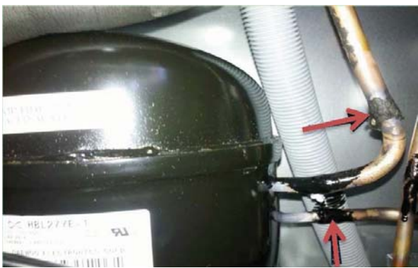
C. Unscrew the compressor.
