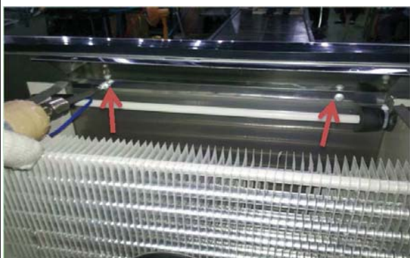
K.Unscrew evap air guide.
