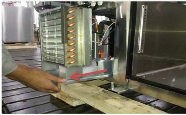
E. Disassembly the condensing unit
