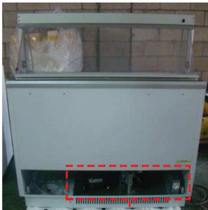
Photo 10 - Machinery compartment view of model TIDC-47W
