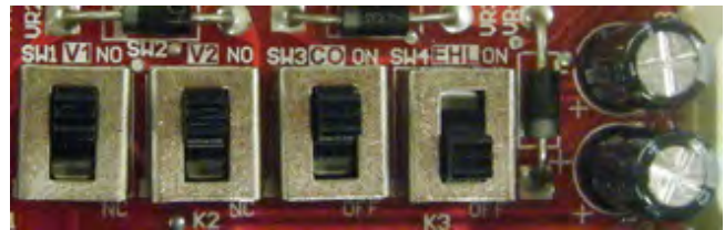
Figure 41. CSTI board-mounted switches
