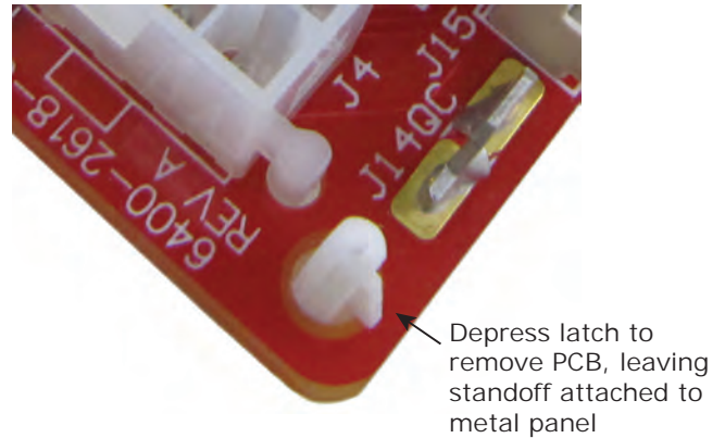
Figure 98. Remove PCB
