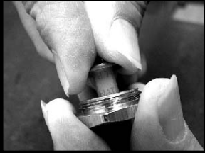
5. Flip the plastic part over & snap the plastic part onto the brass cap in the opposite direction
