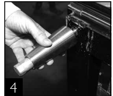
4 Thread leg into cabinet bottom frame rail.
