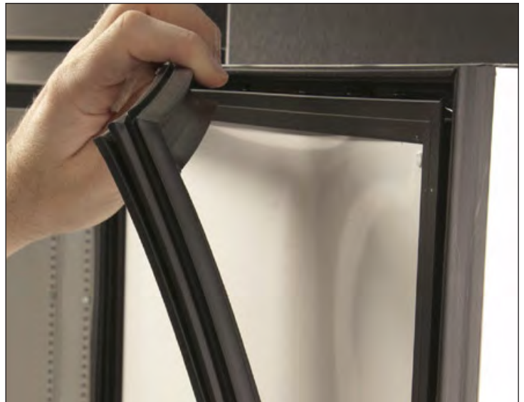
Fig. 2. Pull the gasket starting at an upper corner.
