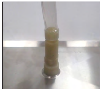
Fig. 5. Hose installed on spill tray tube.
