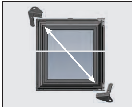
Fig. 5. The current bottom door bracket will be the new top door bracket.
