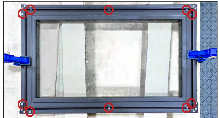
Fig. 7. Cabinet door predrilled hole locations.
