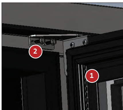
Fig. 10. Install the top hinge and the door.
