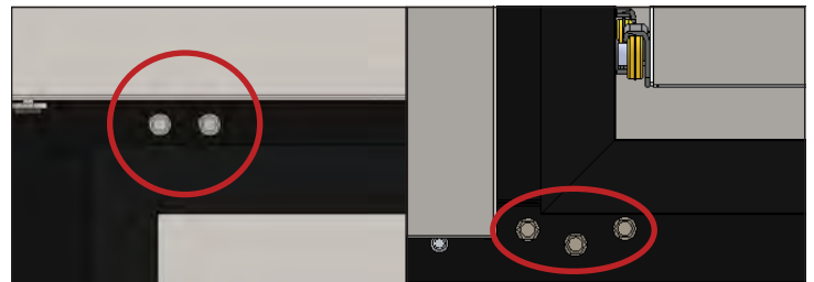
Fig. 4. Remove the remaining hardware from the top and bottom of the appliance on the opposite side of the door opening.
