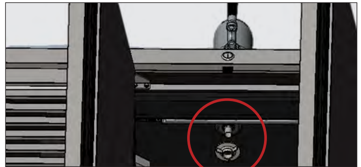
Fig. 1. Spill tray tube nut installation location.
