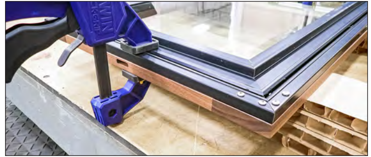
Fig. 6. Be sure the overlay's center slot is positioned at the top of the door.
