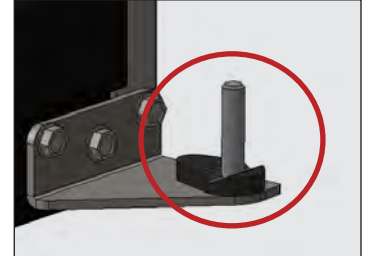
Fig. 3. Lift the door off the bottom hinge.
