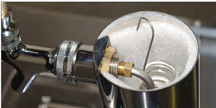
Fig. 8. Hang the chill hose clip over the beer line.
