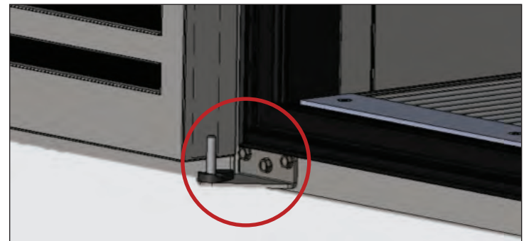
Fig. 3. Lift the door off the bottom hinge.
