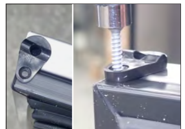
Fig. 6. Install the cam riser on the bottom of the door on the opposite side of its original location.
