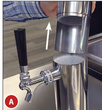
Fig. 7. Route the air hose through the draft tower from below.
