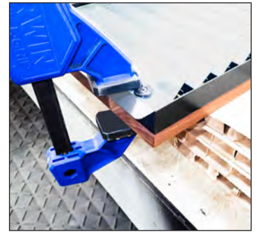
Fig. 2. Center the overlay and grill at the corners. The panel is slightly larger than the grill.
