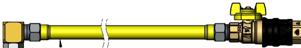
3/4" NPT x 48" [1219mm] Coated Gas Connector w/ SAFE-T-GUARD Quick Disconnect Valve & SwiveLink Fitting
