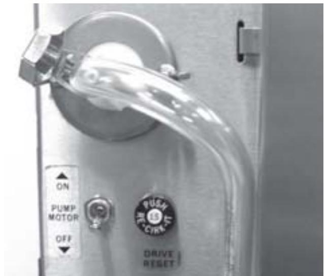
**Figure 3. Pump Controls**
