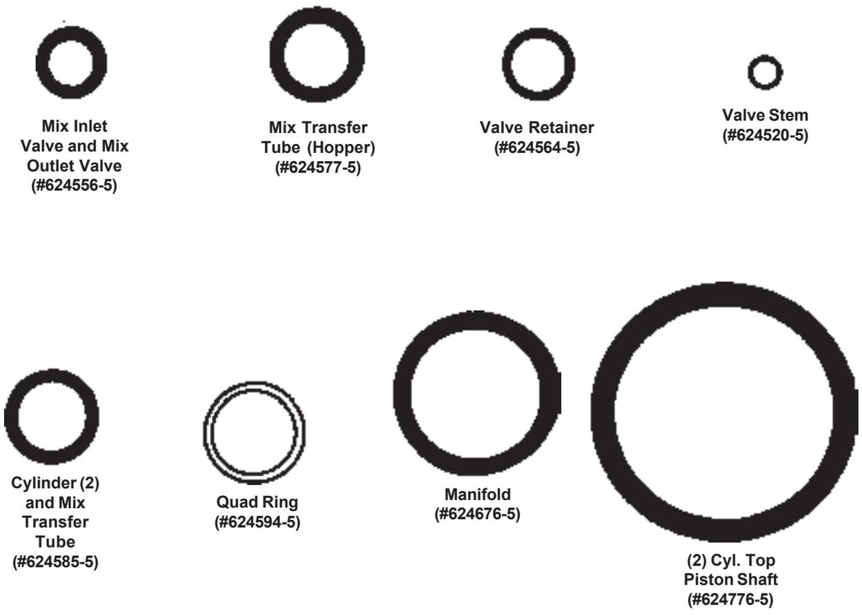
Figure 13. "O"-Ring Identification (Actual Size)
