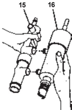
**Figure 8. Pump Disassembly Step Two**
