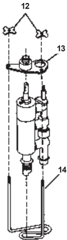
**Figure 7. Pump Disassembly Step One**
