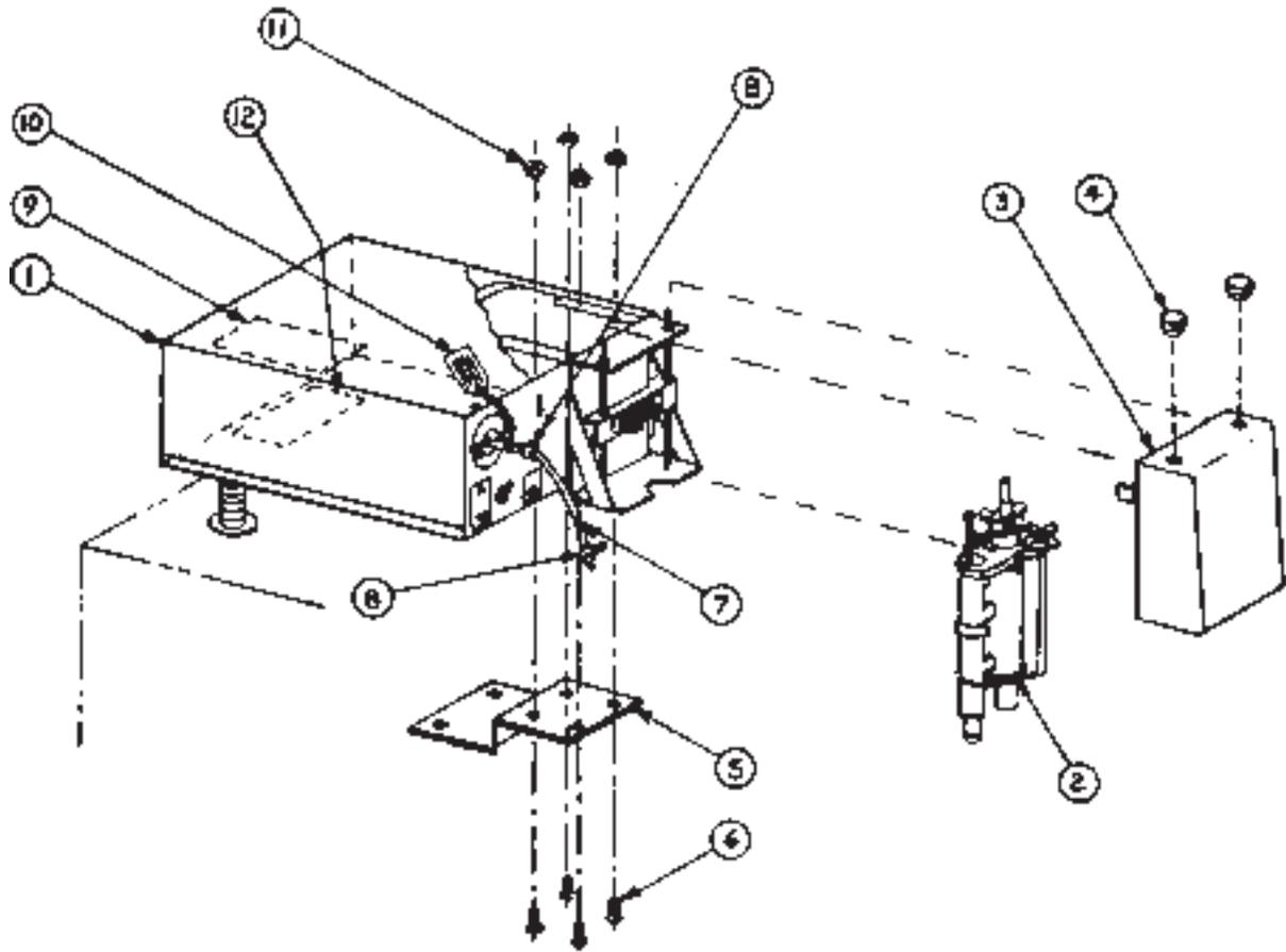
Figure 16. Hopper Pump Final Assembly
