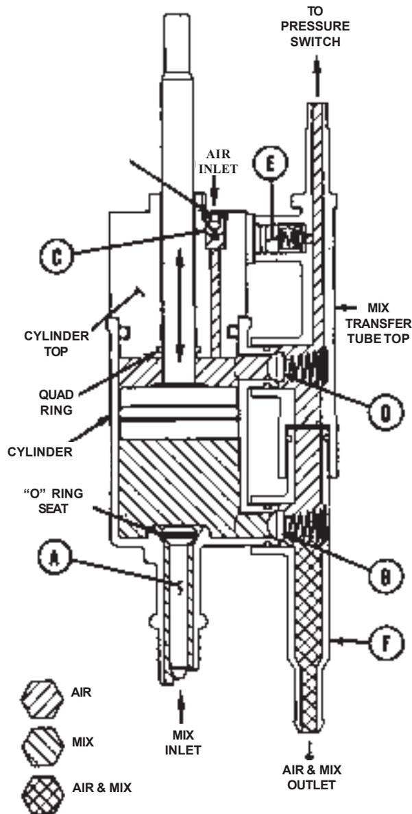
Figure 4. Pump Operation
