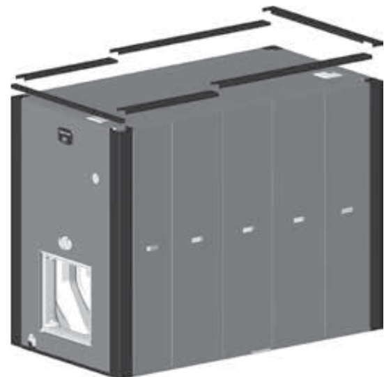
Figure 33 Press jacket trim down over jacket front, rear and side panels
