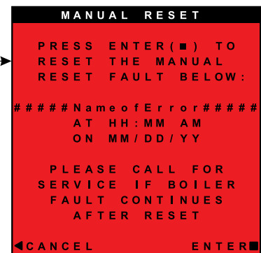
Figure 6 SlimFit boiler control display LOCKOUT SCREEN — screen turns red when boiler locks out — highlight and select MANUAL RESET to reset boiler as shown below.
