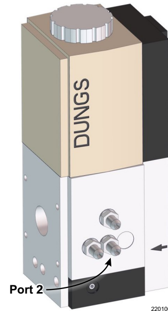
Figure 41 Gas valve pressure test port - SVF 2500-3000
