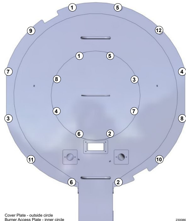
Figure 79 Tightening sequences – SVF 1500-3000
