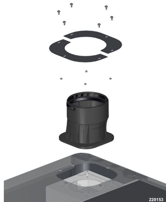
Figure 10 Air inlet 3-1 adapter with cover plates
