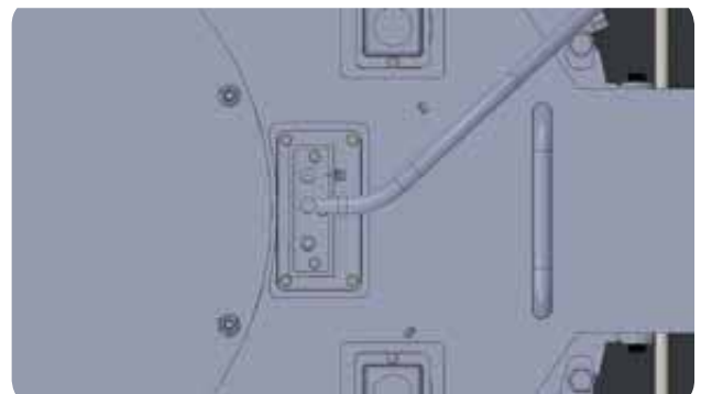
Figure 86 Correct orientation of ignition electrode / flame sense rod sight glass in down position.
