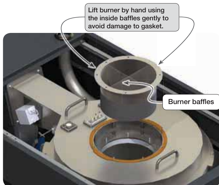
Figure 89 Burner removal and replacement position
