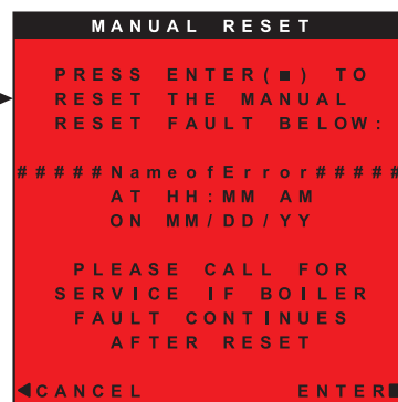
Figure 6 SVF™ boiler control display LOCKOUT SCREEN — screen turns red when boiler locks out — highlight and select MANUAL RESET to reset boiler as shown below.
