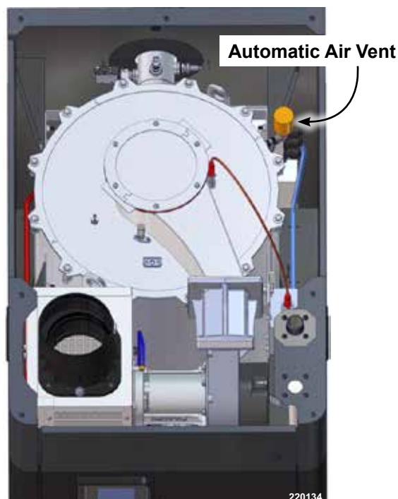
Figure 12 SVF 1000-3000 automatic air vent location
