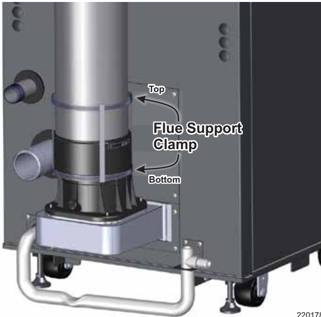
Figure 21 Flue support clamp, installed
