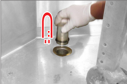
Lift out Drain Stand Pipe.
