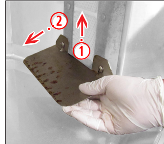
Lift up and pull out the two IR Burner Reflectors.
