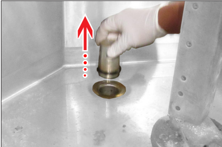
Lift out Drain Stand Pipe.
