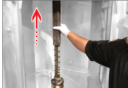
Lift Flame Post Guard completely off Flame Post Burner
